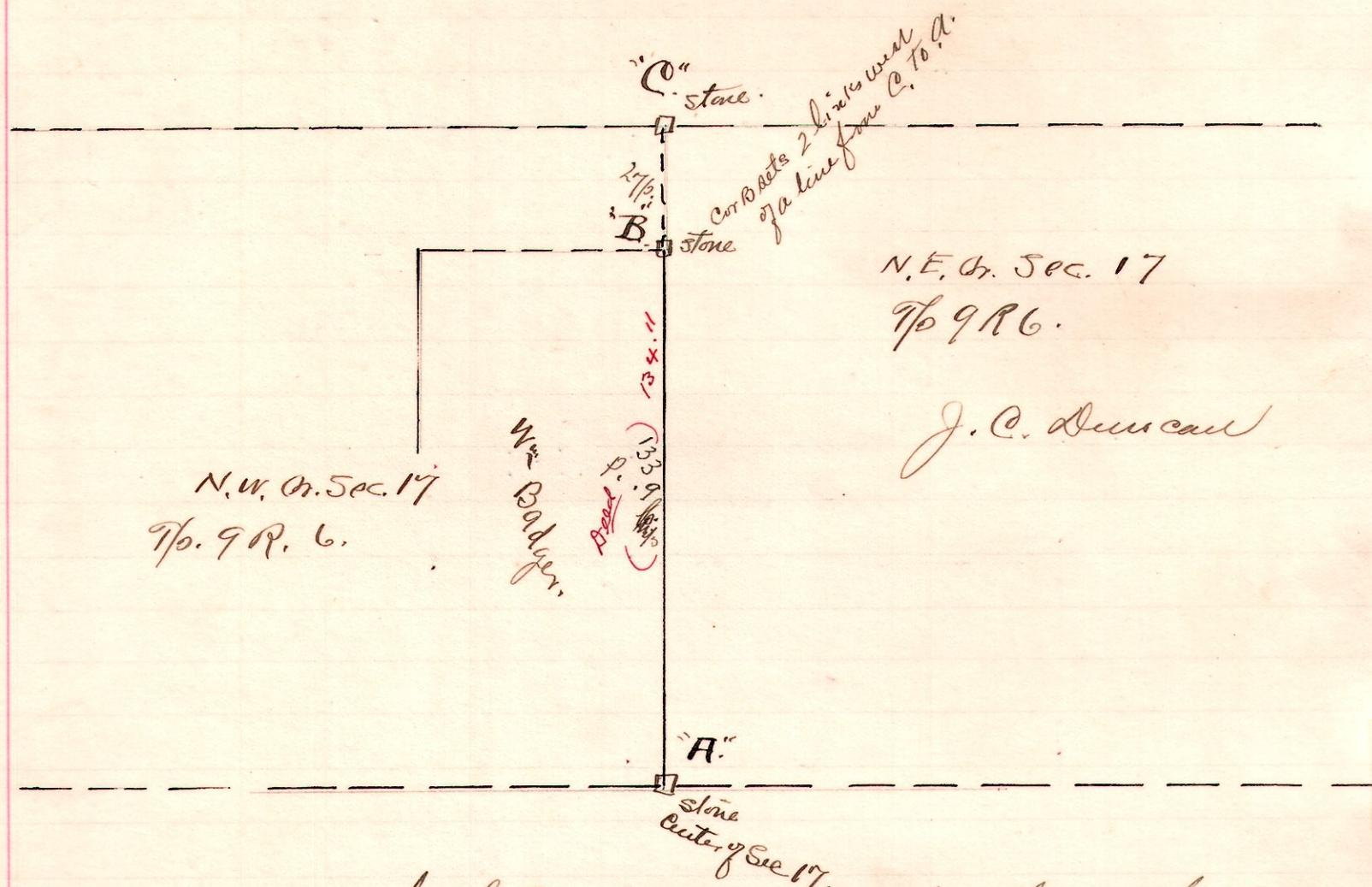
A survey made for the Trustees of Hardy P. to locate the true line A to B. being a division line between lands of J.C. Duncan on the east and W. Badger on the west
